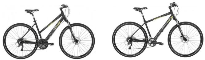
Spanish made BH bicycles (model Silverlite). They are light weight aluminium hybrid bikes with Shimano components and disc brakes front and back. All bikes have a rear carry rack (without panniers) and a front waterproof carry bag that connects to the handlebars (not displayed).
