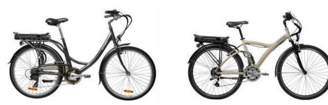
E-Bikes are 24v and 36v battery bikes – hybrid style and they have a rear carry rack (no panniers) and a front carry bag. The batteries are rated for 60 km / day on economic power use and our tours cannot guarantee a spare battery during day riding for every person.
